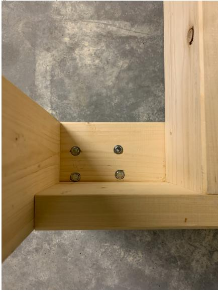
Leave room to drill holes for securing the locking, castering wheels to the forward and aft assemblies.
